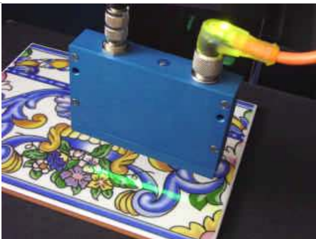
Detection of fluorescent lines on ceramic tiles
