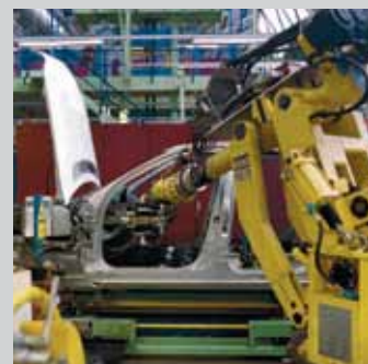
Car production Positioning the body using distance sensors
